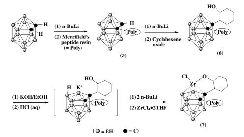
Scheme 2. Synthesis of Merrifield's peptide resin-supported constrained-geometry zirconacarborane.
