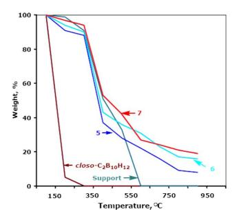
Fig. 2. TGA curves of Merrifield's peptide resin (support), closo- $C_2B_{10}H_{12}$ , 5, 6 and 7.
